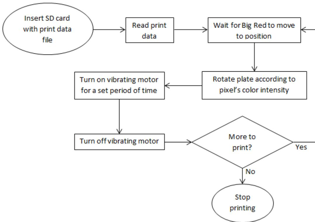
Figure 9. Flow chart of printing process.
