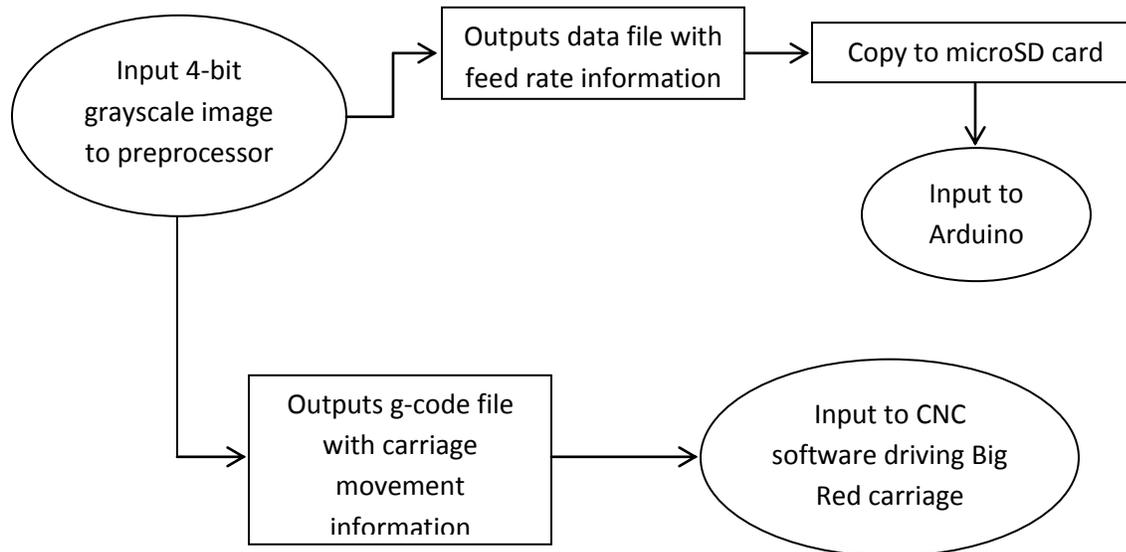
**Figure 10.** Flow chart of preparation process.
