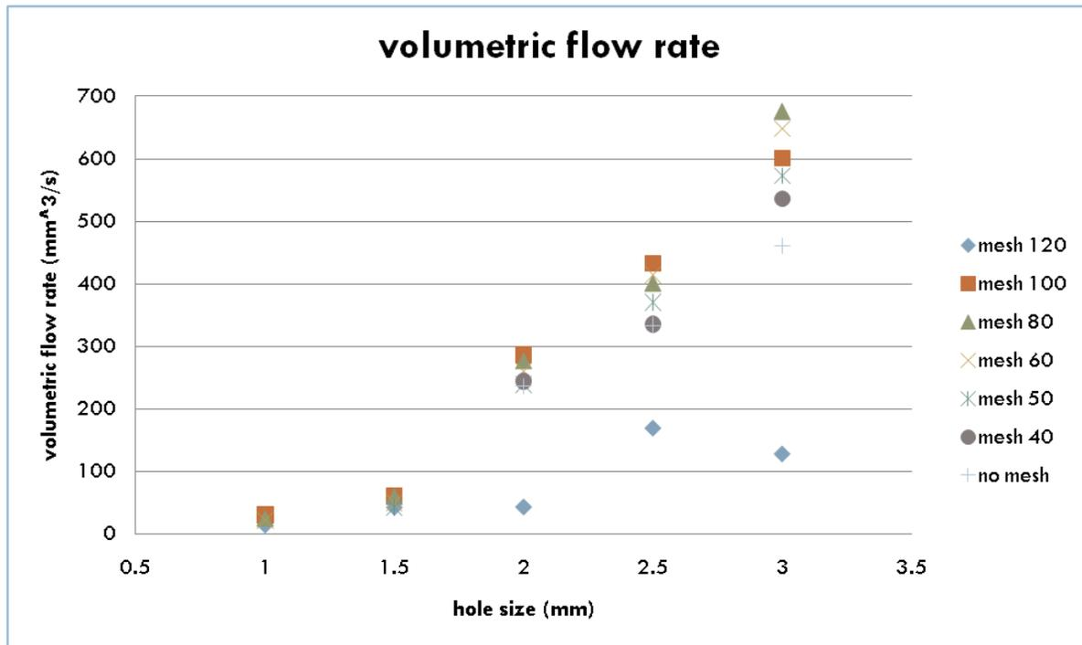
Figure 2. Volumetric flow rate as controlled by hole diameter.
