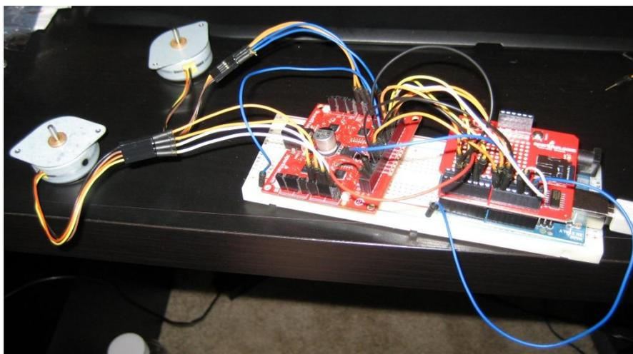
**Figure 11.** Flow rate control hardware.
