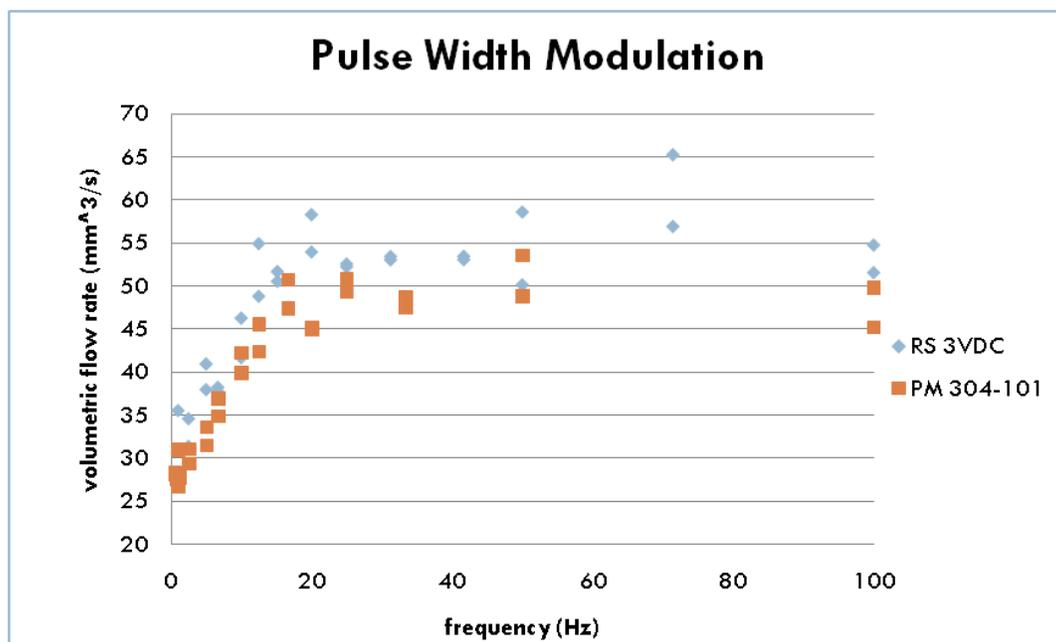
**Figure 1.** Flow rate control using pulse width modulation.
