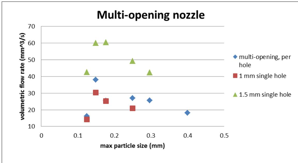
Figure 3. Effect of multiple holes per nozzle.
