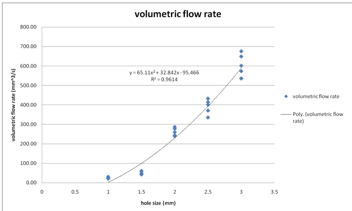
**Figure 18.** Volumetric flow rate as a function of hole size.
