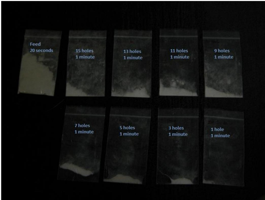
**Figure 17.** Powder deposited for different hole densities.
