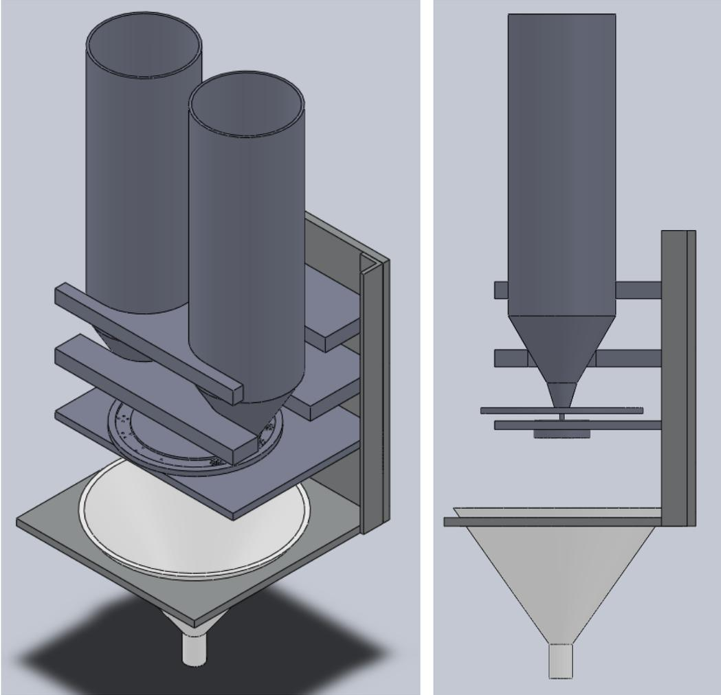
**Figure 7.** Powder print head assembly.
